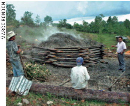
Traditional charcoal making in Lempira, Honduras, has changed little over the years. A modern pyrolysis plant could produce energy as well as biochar more cleanly.
