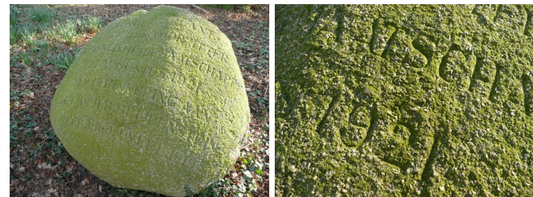
Figure X: Weathering of granite memorial stone, Judithhoeve, Losser (NL)
