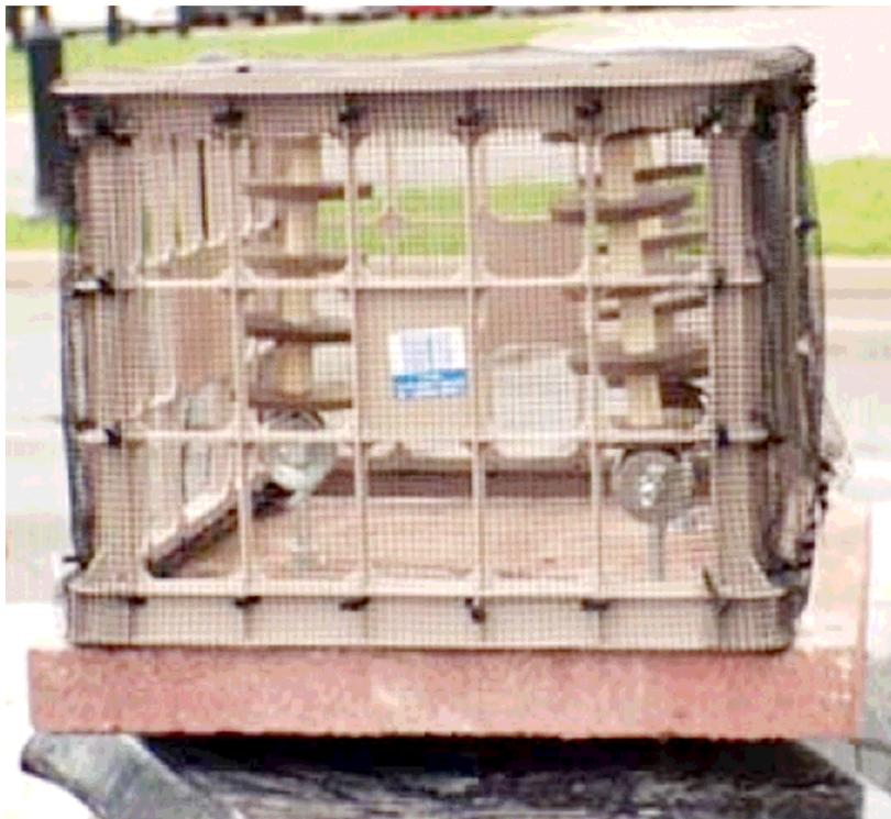
**Figure 3.** Open (top) and screened (bottom) Hester-Dendy artificial substrate sampler units for the macroinvertebrate colonization experiment.
