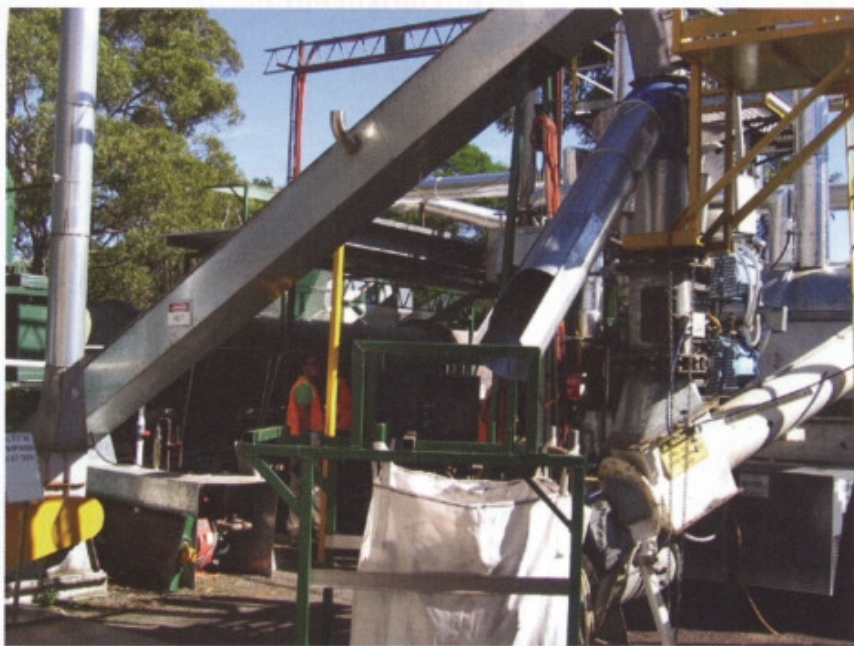
BEST ENERGIES' BIOMASS BAKER Pyrolysis can be fine-tuned to maximize the yield of either usable gas as an energy source or charcoal for agriculture. Yet by not optimizing the baking process to favor either at the expense of the other, well-balanced pyrolysis can do more for the health of the earth.
