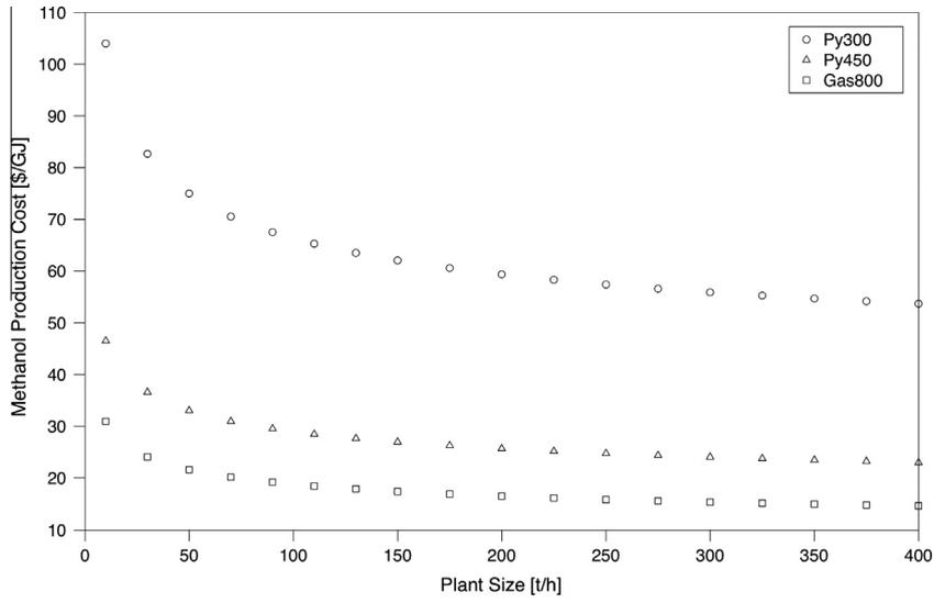
Fig. 2. Methanol production costs in relation to plant size.
