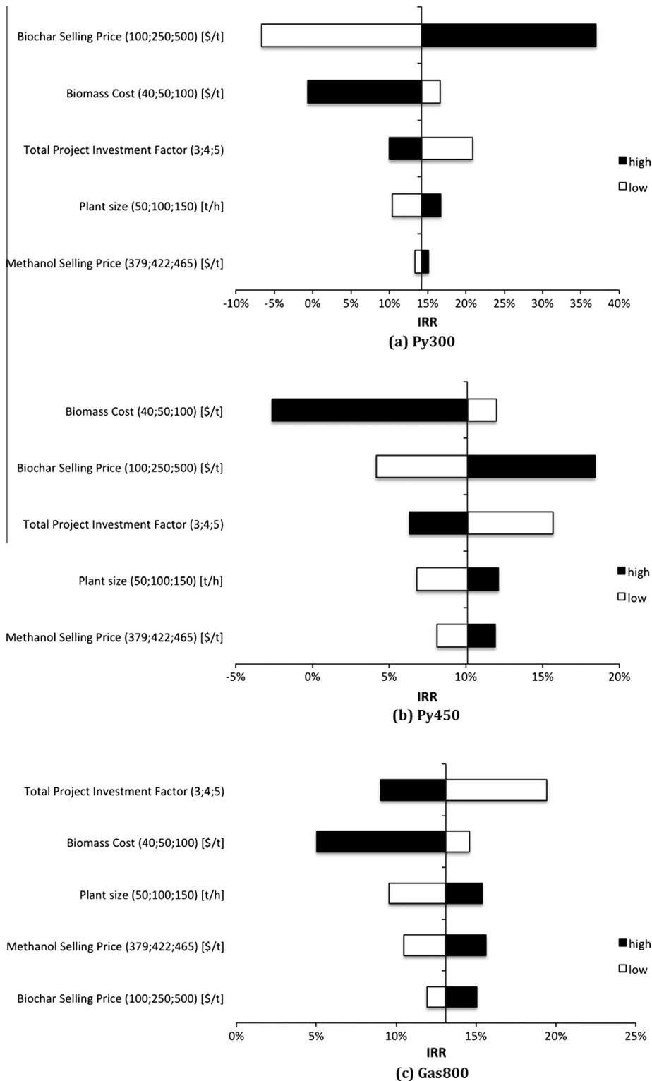
Fig. 4. Sensitivity analysis for a plant size of 100 t/h for (a) Py300 (b) Py450 and (c) Gas800.
