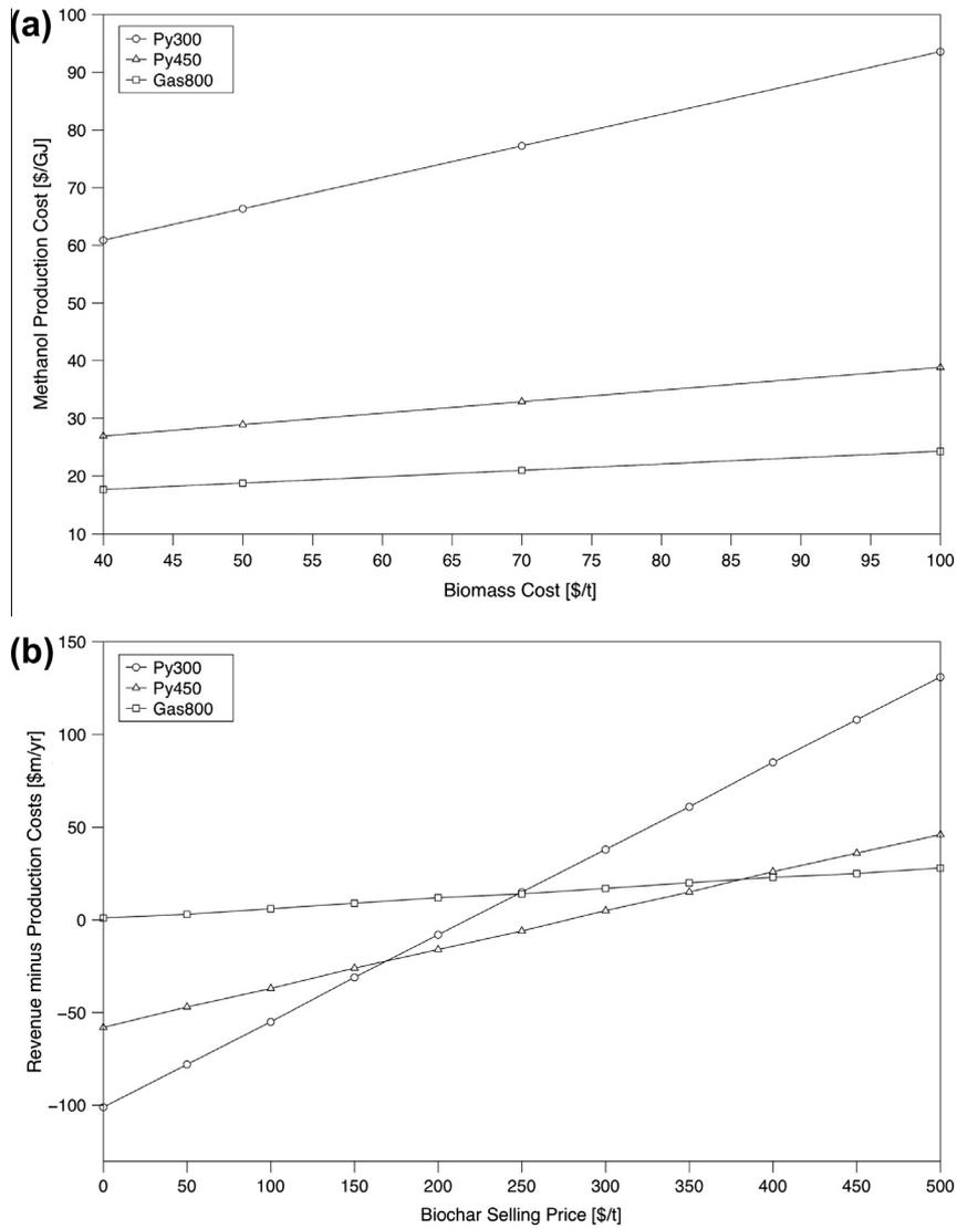
Fig. 3. (a) Methanol production costs in relation to biomass cost and (b) Profitability in relation to biochar cost, for a plant size of 100 t/h.
