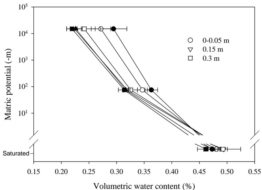
**Supplemental Fig. S1. Soil moisture retention curves for samples taken at various depths from plots receiving 0 (open symbols) or 20 t biochar ha<sup>-1</sup> (closed symbols) (n=4).**
