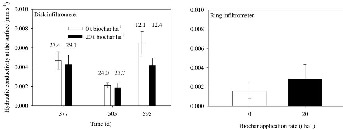
**Supplemental Fig. S2. Surface hydraulic conductivity measured with a disk infiltrrometer (left panel,  $\pm$  SE,  $n=12$ ) and a double-ring infiltrrometer (right panel,  $\pm$  SE,  $n=3$ ) on a Colombian savanna Oxisol during the fourth year after biochar application. Numbers above bars show the surface soil's percent volumetric moisture content at the time of measurement.**
