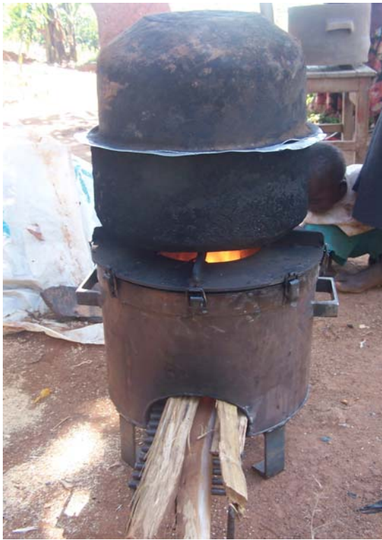
Figure S3. First generation pyrolysis stove and cross sectional diagram
