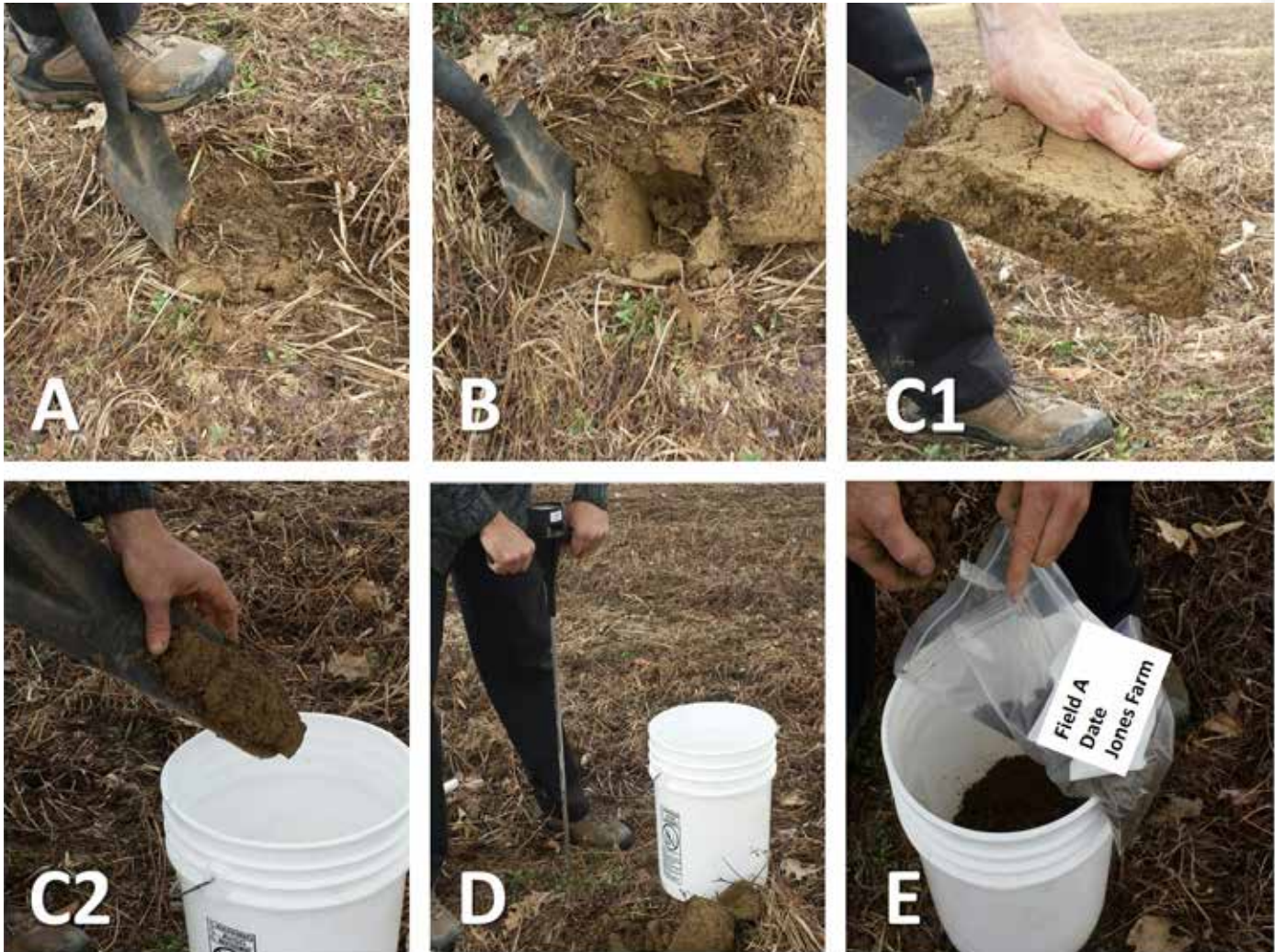
FIGURE 2.11. The steps of taking a soil health sample. The microorganisms in the soil are sensitive to heat. Keep samples out of the direct sunlight and keep as cool as possible during the sampling. Store samples in a refrigerator or cold room after returning from the field and ship to Cornell as soon as possible. Photo credit: Kirsten Kurtz
