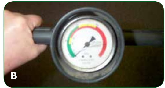
FIGURE 2.18 A and B. Measuring surface and subsurface hardness with a penetrometer.
