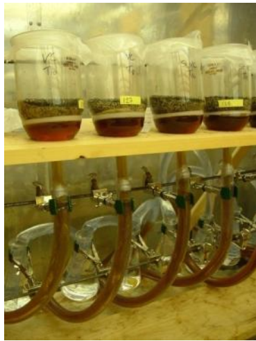
Figure 4. Apparatus for controlling matric potential for disease suppressive bioassays. Fritted glass Buchner funnels being passively watered through gravity on a water column under vacuum.
