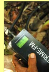
Figure 2. Measuring volumetric water content using TRIME-FM (IMKO GmbH)
